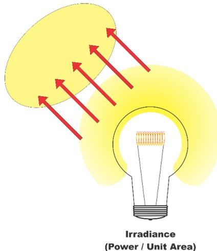
Figure 13 is a graphic showing the output of a light source and its irradiance on a unit area.
