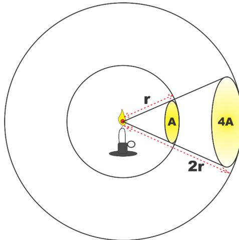
In the center we have our light source, in this case a candle. “A” is the unit beam area at a distance of radius “1r”. At 2r, the beam area increases by a factor of 4 **BUT the intensity is subsequently reduced by a factor of 4!**
