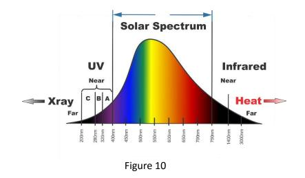
Figure 10 represents the portion of the EM spectrum emitted by the sun known as the solar spectrum of light also referred to as solar irradiance. In the above figure, to the left of the visible spectrum is the UV (ultraviolet). This is the light (invisible) that causes sun burn and skin cancer. To the right, we transition into the IR (infrared) which we feel as heat. A more precise chart of solar irradiance is shown if figure 11.
