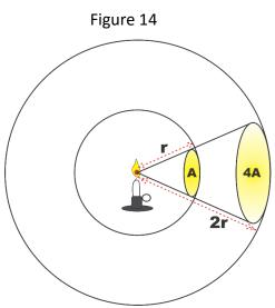
In the center we have our light source, in this case a candle. "A" is the unit beam area at a distance of radius "1r". At 2r, the beam area increases by a factor of 4 **<u>BUT</u>** the intensity is subsequently reduced by a factor of 4</u>!
